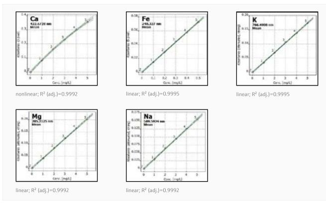
Figure 1: Resulting calibration functions and correlation coefficients
