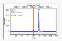
Figure 9: Spectrum of Ni in sewage sludge 2 corrected with IBC
