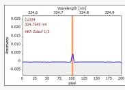
Figure 8: Spectrum of Cu in inlet wastewater corrected with IBC
