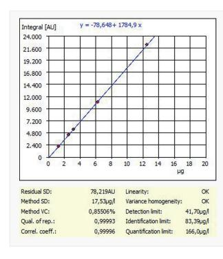
Figure 1: liner regression and method characteristics for TOC calibration
