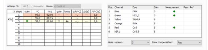
Figure 3: Overview of the settings for *Legionella* detection in qPCRsoft for the real-time PCR on the qTOWER<sup>3</sup>. *Legionella pneumophila* and *Legionella spp*. can be detected in the blue and red channel, respectively. In the green channel the internal control can be detected.
