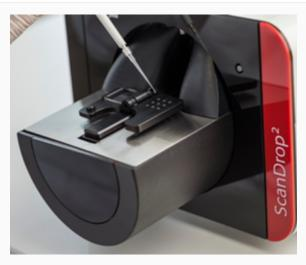
Fig. 2: Filling the Butterfly Cuvette
